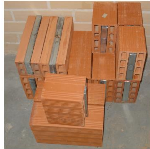
Clay bricks with PCM macrocapsules (Silva et al.)
