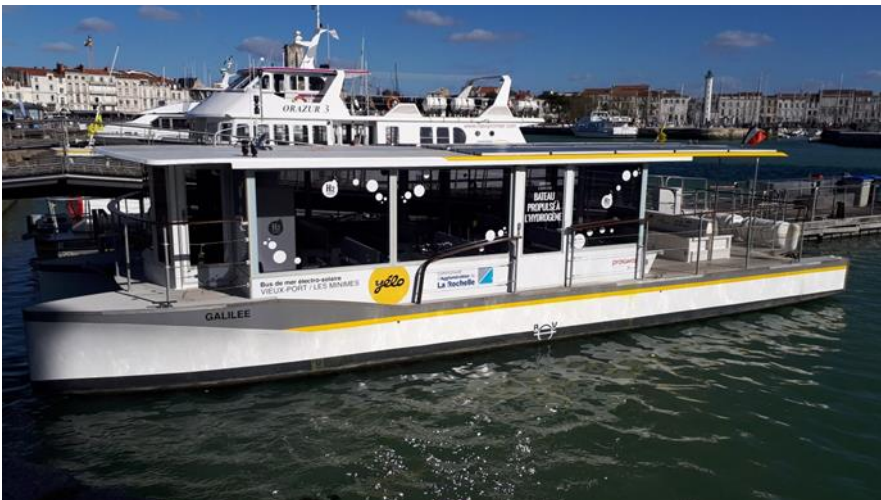
H 2 water bus, "Alternatives Energies" La Rochelle, France
