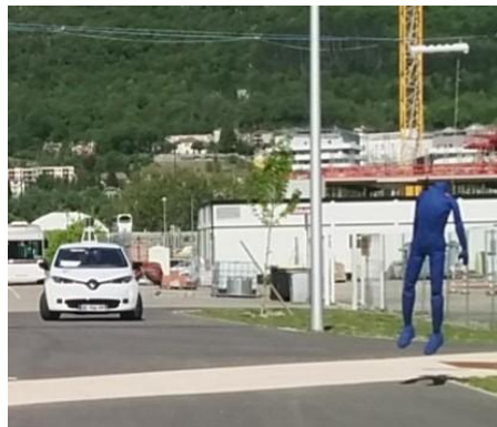
Equipment for pedestrian crash test
